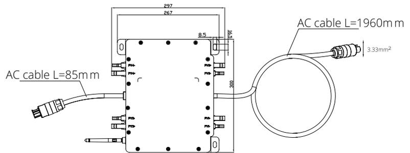
The AC wire on the micro inverter is a TC-ER wire with a wire cross-section area of 3.33mm<sup>2</sup>.
