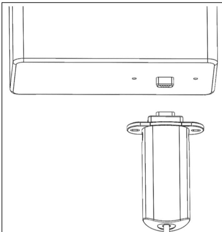
Insert the two screws that come with the Data Logger through the holes, and then tighten them with a Phillips screwdriver, as shown in the figure below.
