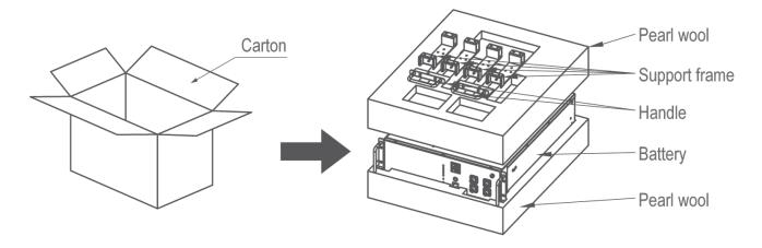
After unpacking the battery, check whether deliverables are intact and complete. If any damage is found or any component is missed, contact the dealer.
